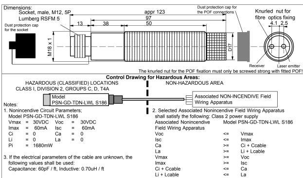
4. Power, input and output (I/O) wiring must be in accordance with Class I, Division 2 wiring methods - Article 510 - 4(b) of the NEC/NFPA 70or as specified in Section 18-152 for installation within Canada and in accordance with the authority having jurisdiction
