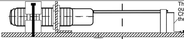
The end of the cable must be connected outside the hazardous locations. Check the reliable, noncorrosive holding of the protection earth connection.
